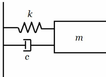
**Figure 7:** Mass spring damper schematic
