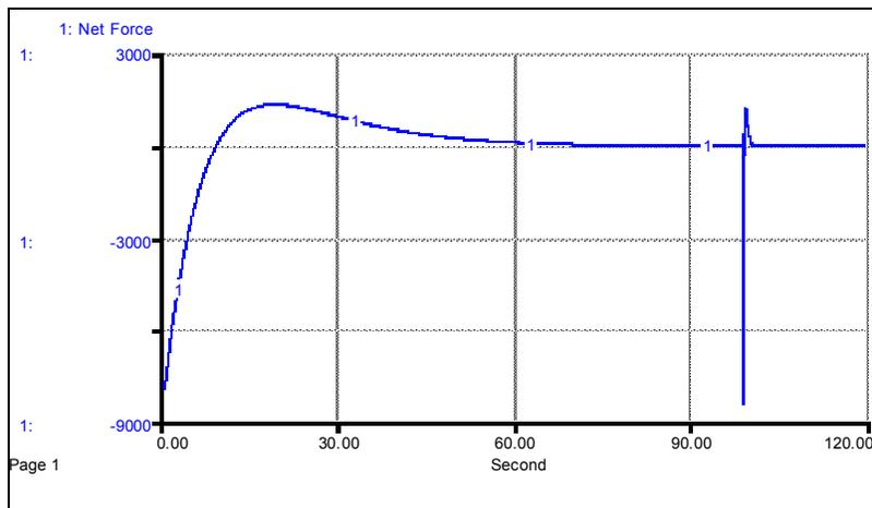
**Figure 5:** Net force acting on the vehicle during landing
