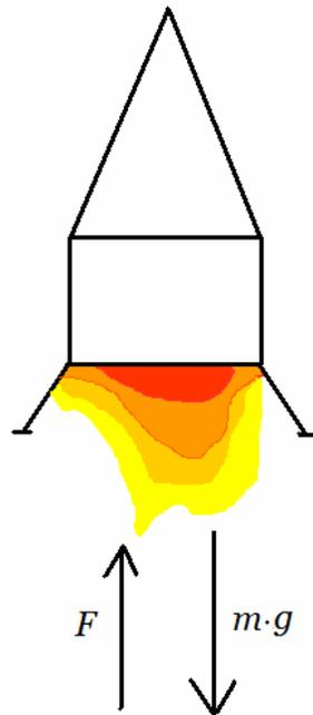
**Figure 1:** Free body diagram of the vehicle with a control force ( $F$ ) generated by the reverse force thruster and the gravitational force ( $m \cdot g$ )
