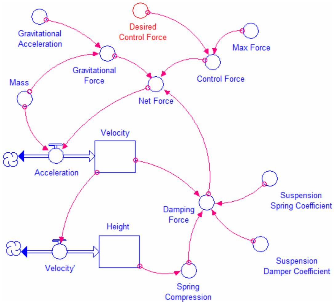
**Figure 2:** Stock-flow diagram of the model
